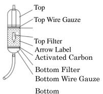
2. Take out top wire gauze, top filter, activated carbon, and bottom filter.
