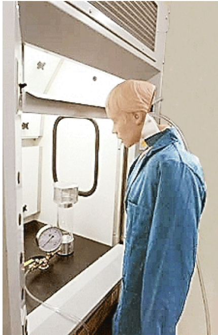
ANSI/ASHRAE 110 Method of Testing Performance of Laboratory Fume Hoods
