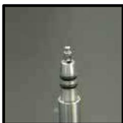
Daub a matrix mixed sample on the probe tip.
