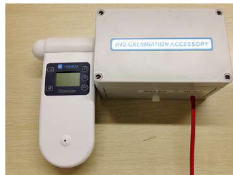
Use this orientation for calibrating CO
