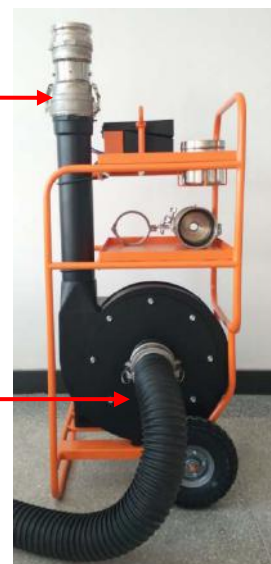
High flow Duct testing under Negative pressure
