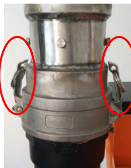
Cam lock adaptor in locked status.
