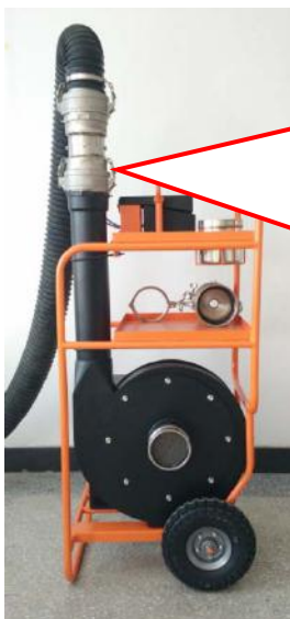
High flow Duct testing under positive pressure
