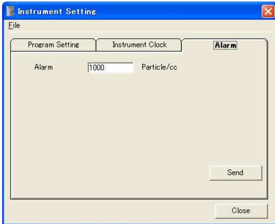
Alarm setting: Sets an alarm value of the CPC.
