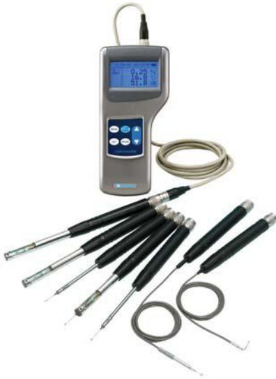
Climomaster shown with all the available probes
