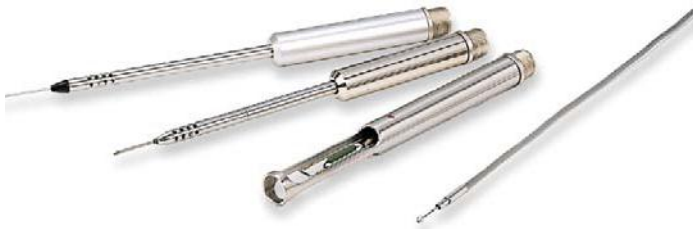
Four common types of hot-wire probes
