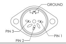
Mating Cable Connector: Switchcraft Part No. 05CL3MX (RoHS version) Switchcraft Part No. 05CL3M (non-RoHS version)
