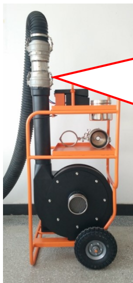
High flow Duct testing under positive pressure
