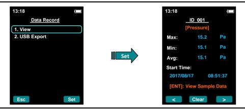
Click " < " or " > " for reviewing the statistic value of differential pressure, air velocity and airflow.
